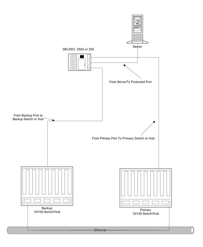
The Implementation of either an SM-2501, SM-2500, or SM-250 for a single protected port, in a copper based LAN environment. The SM-250 for 10BaseT applications only and the SM-2500 for 100BaseTX only. The SM-2501 is autonegotiate with programmable swithover times. Each device is equipped with an audible alarm for notification on failover
