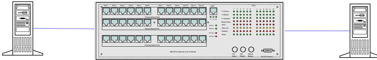
Server Farm with Copper NIC's using SM-2512 to Create Redundancy Building One Floor X
